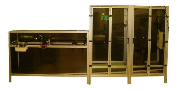
Impact speeds in tennis can be very high. For example, in a smash, the ball can hit the court at over 180 km/h (112 mph). To simulate the effects of high-speed impacts in tennis we use a 'bazooka' air cannon that is capable of firing a ball at this speed. This equipment can be set up to model the impacts between balls and both rackets and surfaces.
