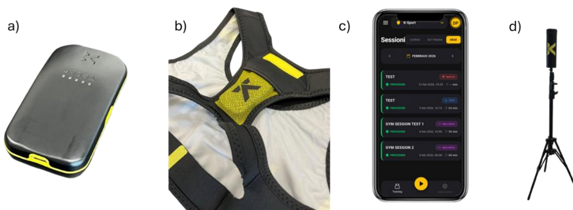
Figure 1 - Components of the System: a) The device removed from the harness; b) the device placed in the harness to be worn between the shoulder blades; c) the smartphone app; d) the courtside antenna for optional LIVE data transfer.
