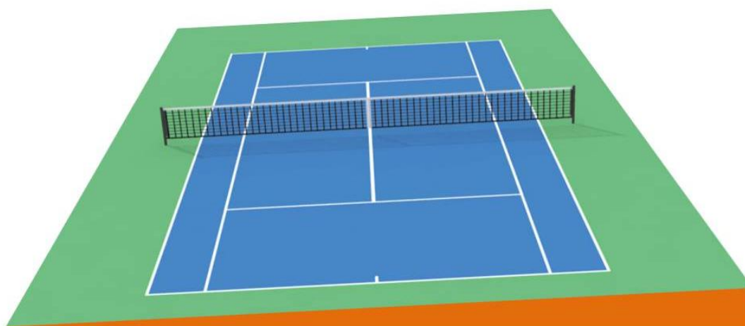
Figure 6. Preferred orientation of slope (side-to-side), if necessary.
