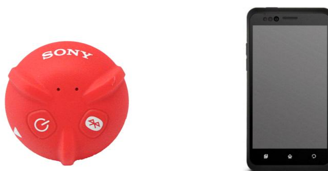
Figure 1. Components of the SONY Smart Tennis Sensor system: Smart Tennis Sensor pod (left); auxiliary device (smartphone).
