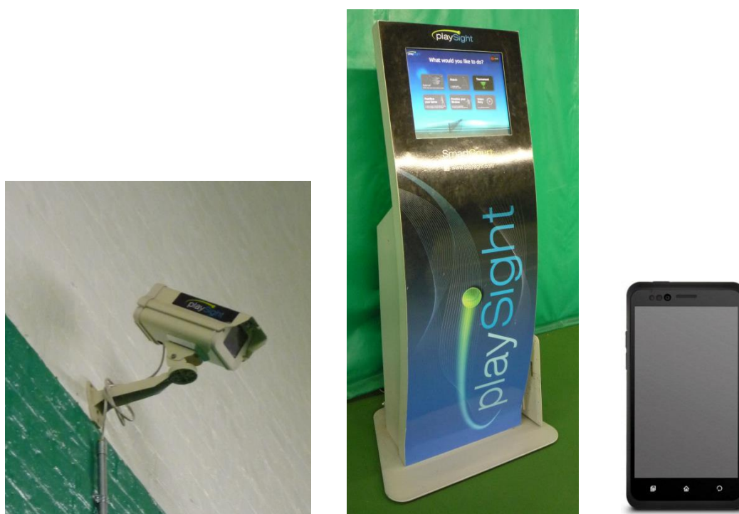
Figure 1. Components of the PlaySight SmartCourt system (from left to right): video camera; on-court kiosk; auxiliary device (smartphone).
