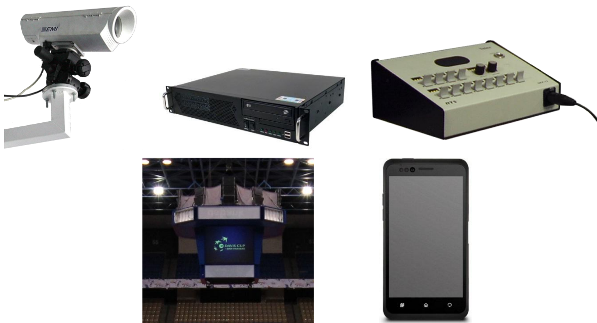
Figure 1. Components of the Hawk-Eye system (from left to right): Video camera; PC; two-way radio (talkback panel); in-stadium display; auxiliary device (smartphone).
