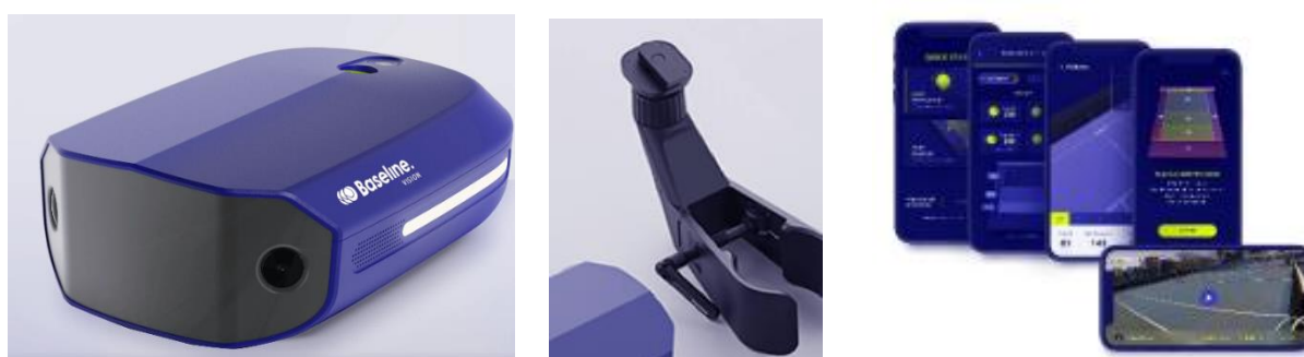
Figure 1. Components of the Baseline system (from left to right): Baseline Vision device (with LED strip illuminating white); Baseline net post mount; auxiliary device (smartphone) showing the Baseline app. Not to scale.
